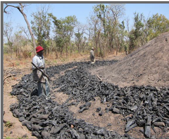
A charcoal kiln in Sare Bidji, partway through transformation. As the tree rounds burn, ready charcoal is raked from the fire to cool in wide rings.
