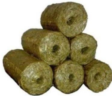
Figure 4: Non carbonized briquette made from straw waste using a piston extruder (middle)
