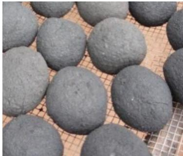
Figure 3: Briquettes made by hand from charcoal waste (left)
