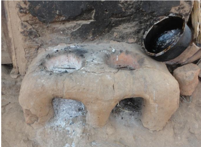
Figure 7-3. Basic improved charcoal stove in Mwamgongo Village, Tanzania.
