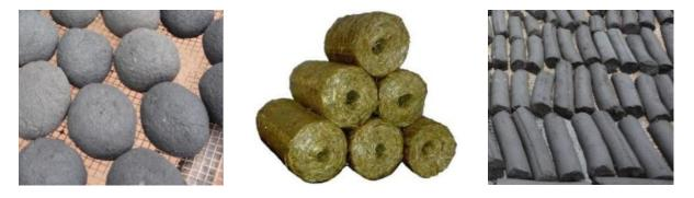
Figure 3: Briquettes made by hand from charcoal waste (left)
