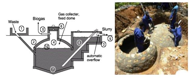
Figure 9: Fixed dome biogas plant (left)
